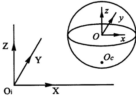
Fig. 4 A sphere rolling on a plane;  $O_i(0,0,0)$ ,  $O(x,y,0)$ ,  $O_c(x,y,-r)$  (where  $r$  is the radius of the spherical shell)
