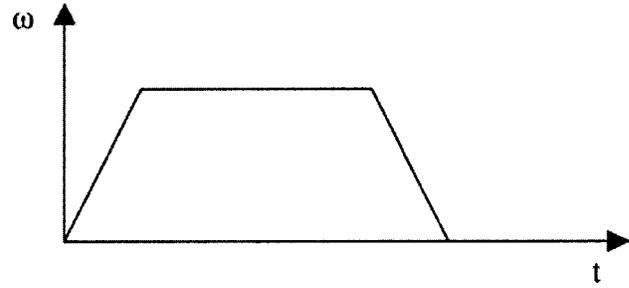
Fig. 5 Angular velocity and time diagram of robot motion, from beginning to destination
