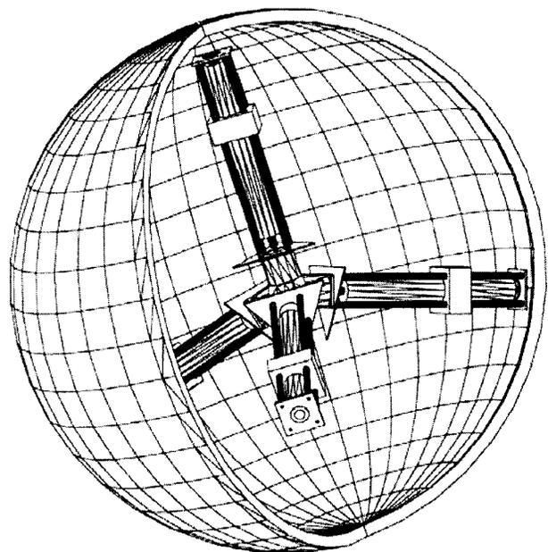
Fig. 1 Inner propulsion system showing whole the system
