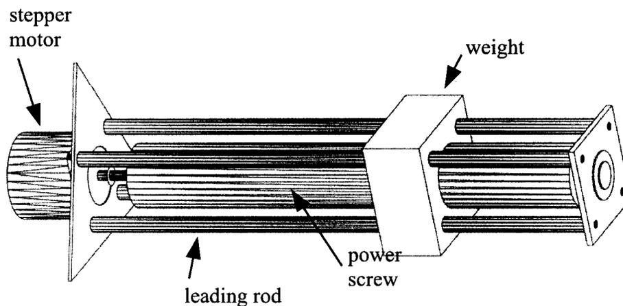
Fig. 3 A closeup of a spoke containing a stepper motor, a cylindrical screw, and a weight
